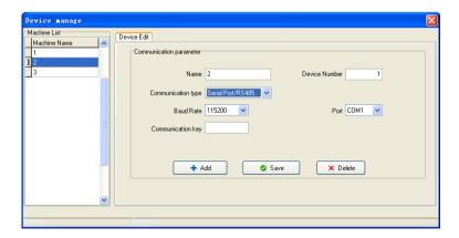
There are two default communication modes provided in the system, one is RS232/RS485, another is Ethernet. Some specify machine is designed with USB communication mode (such as H2), for more detail, please refer to corresponding "User Manual", the using method please view the explanation below:
