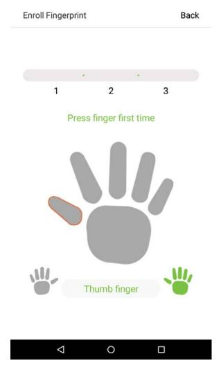
2. Press the same finger on the fingerprint reader three times. Green indicates that the fingerprint was input successfully.
