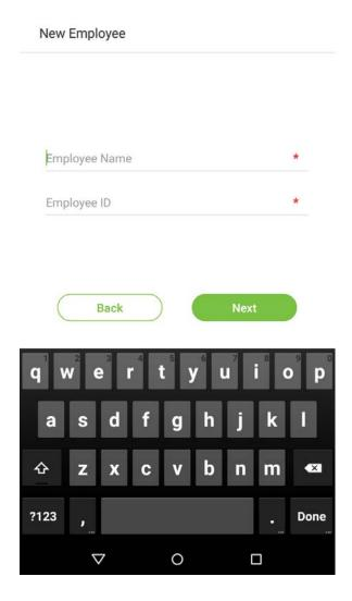
**Note:** This device supports input methods of Chinese, English, numbers, and symbols. Press [CN] to switch to the Chinese keyboard; press [EN] to switch to the English keyboard; press [?123] to switch to the numbers and symbols keyboard; and press [Back] to return to the alphabet keyboard. If you tap on an input box, the virtual keyboard will pop up on the screen. To hide the keyboard, tap on the downwards arrow  $\nabla$ .
